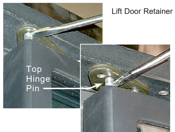
Remove Top Hinge Pin from Top Hinge Socket
